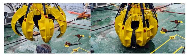
Figure 3.2. Example of a grappler used to remove boulders from the seabed (source: https://www.assogroup.com/)
