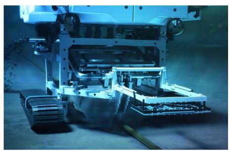
*Figure 3.10.* Jetting equipment example (Source: https://www.youtube.com/watch?v=wblle4zRA2M)
