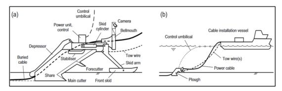
Figure 3.15. Technology of cable line laying using a cable plough (source: https://rules.dnv.com/)
