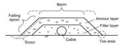
Figure 3.16. Cross-section of a rock dump used for protecting a subsea cable laid on the seabed surface (source: internal materials)
