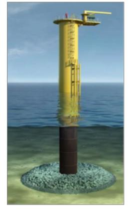
Figure 3.5. Example of a monopile foundation including a scour protection layer (source: Ramboll)
