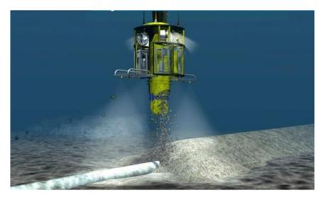
*Figure 3.17.* Visualisation of a rock dump construction (source: www.offshore-fleet.com/data/rock-dumping-vessel.htm)
