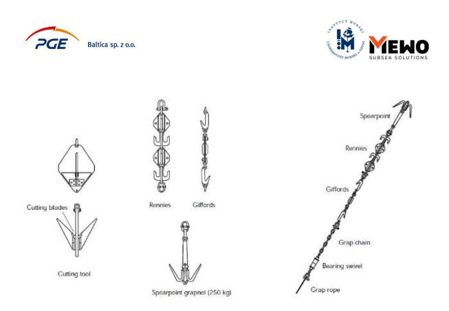
*Figure 3.3. Examples of dragged tools for the seabed pre-lay clearance (source: HKA Submarine Cable -Chung Hom Kok, Project Profile)*
