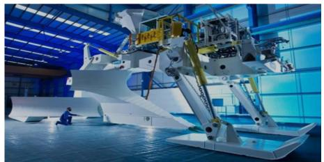
Figure 3.14. Example of a submarine cable plough (source: https://www.youtube.com/watch?v=wblle4zRA2M)
