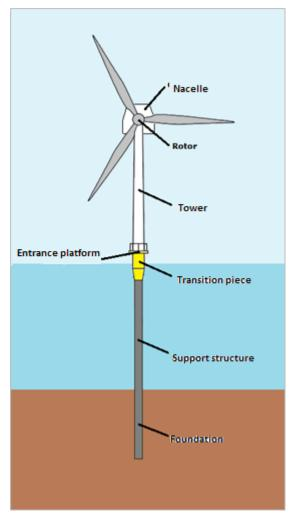
*Figure 3.4.* Schematic diagram of a single wind turbine with an example of a monopile foundation (source: internal materials)
