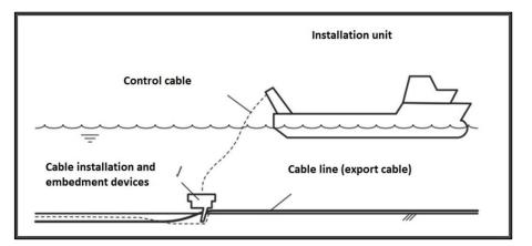
Figure 3.11. Cable line laying technology – burial of a cable previously laid on the seabed (Source: https://rules.dnv.com)
