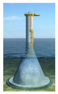
*Figure 3.7. Example of a gravity-based structure (source: Ramboll)*
