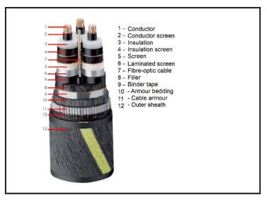
*Figure 3.8.* Design of a typical three-phase AC power cable (Source: internal materials)
