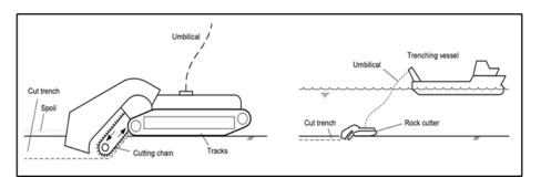
Figure 3.13. Mechanical dredger (source: https://rules.dnv.com)
